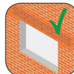
Avoid stress cracking
