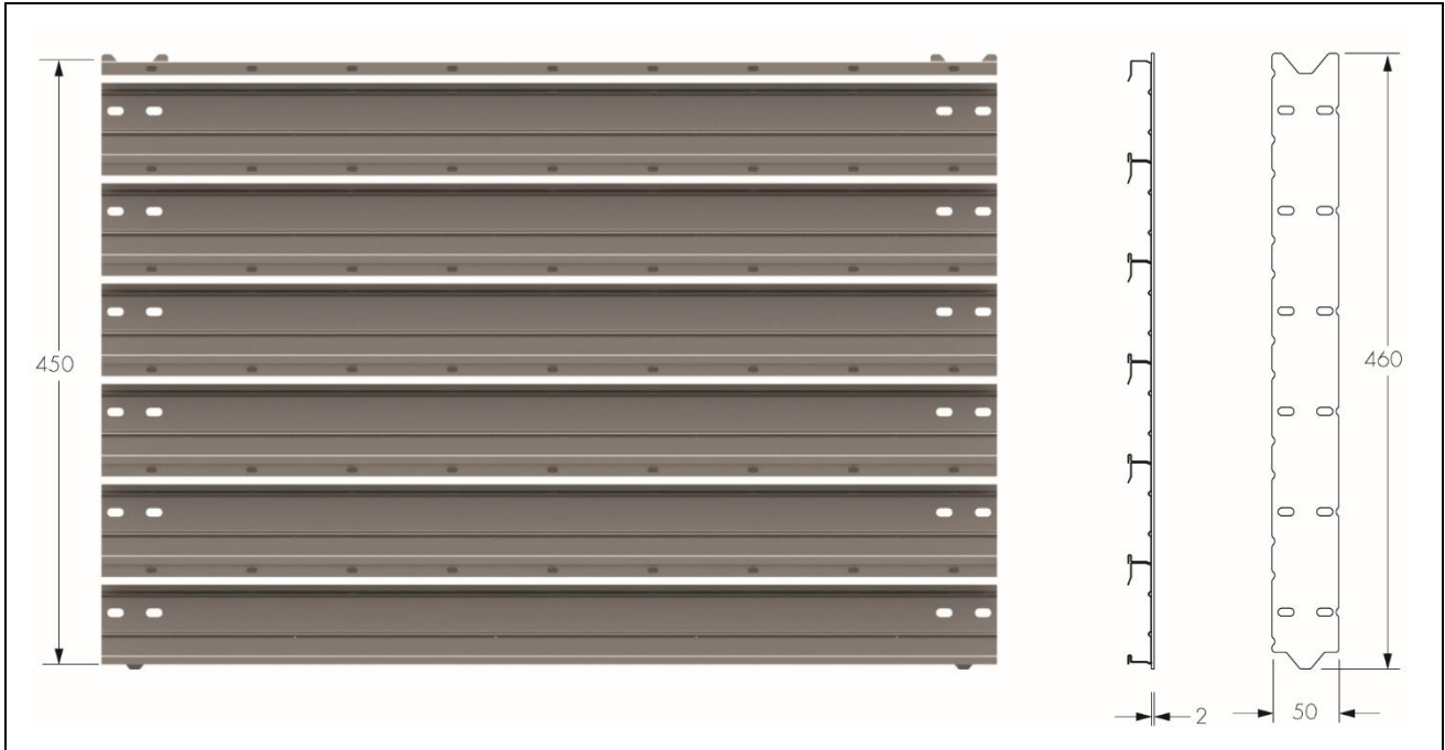
Figure 2 Carrier system – standard panel (measurements in mm)
