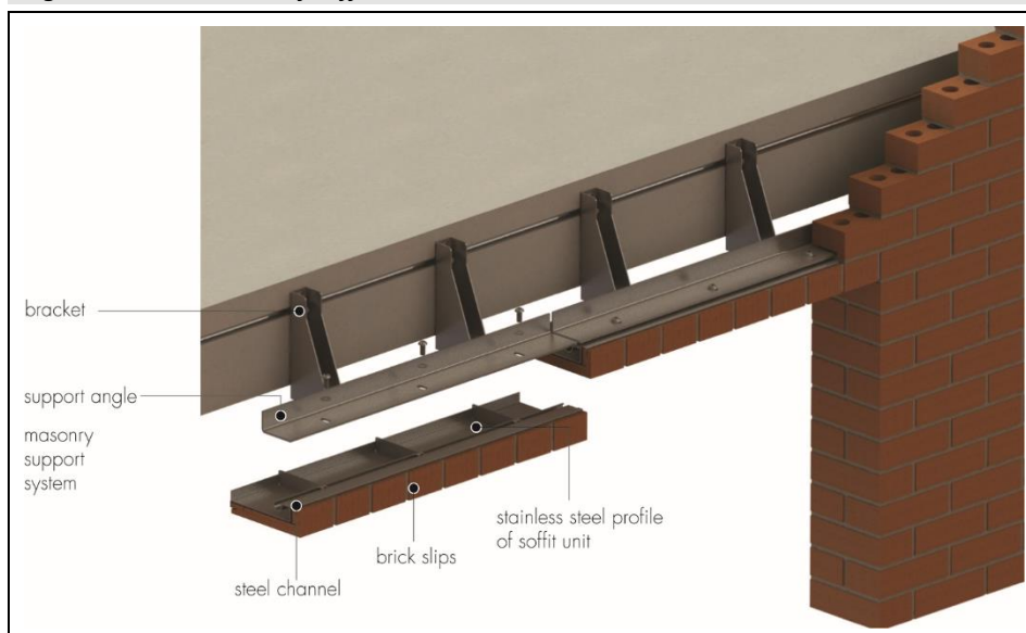
Figure 11 Installation of soffits
