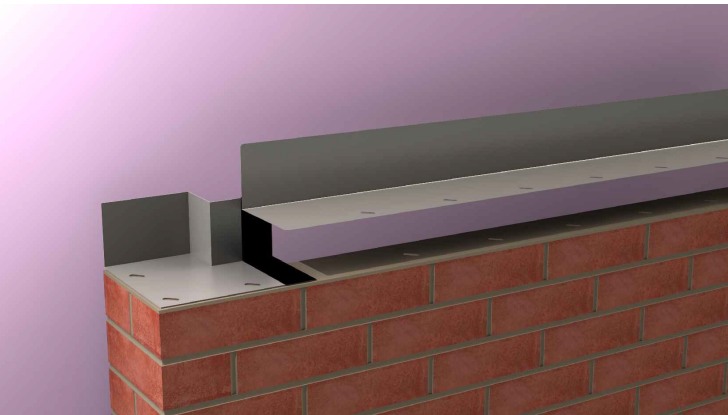
Fig 3. - GT1 double sided tape
