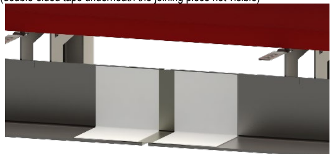
Diagram 4 - Fully sealed angle joint with joining piece and single-sided tape (double-sided tape underneath the joining piece not visible)
