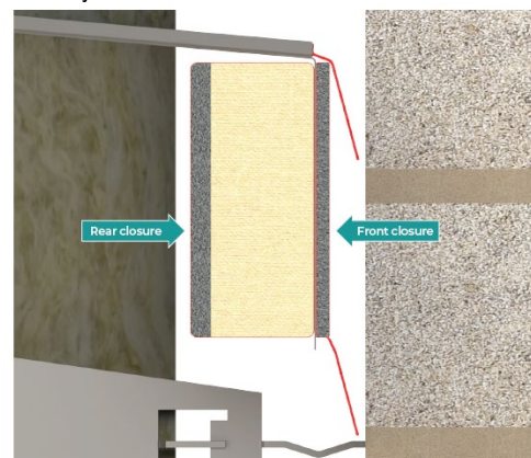
Diagram 2 - Cavity barrier detail
