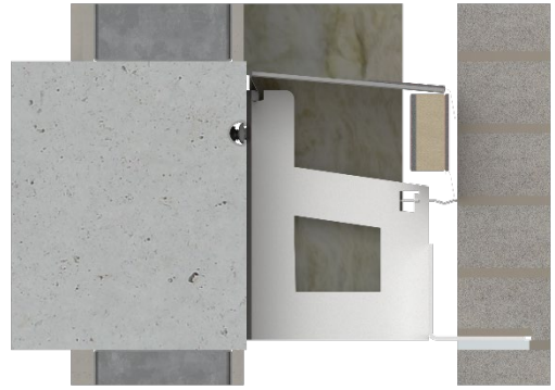
Diagram 9 - Installation with the MW insulation in place (outside the scope)
